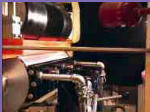
Dow Corning has developed a process which stops misting (left) on release coating lines. Picture right shows solvent release coating running at 700 m/min (2300 ft/min) with 2% Syl-off 7137 High Speed Crosslinker
