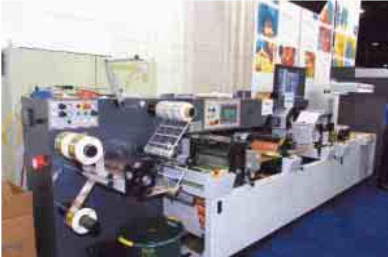
Omega QC330 converting unit on-line with HP ws4000 press
