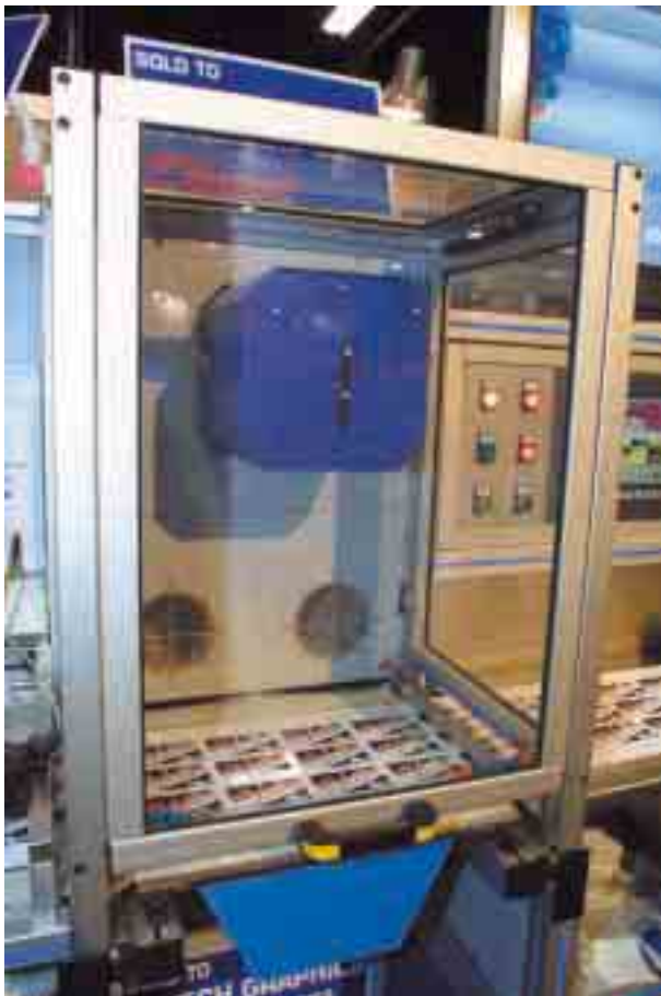
Cartes laser die cutting unit in action
