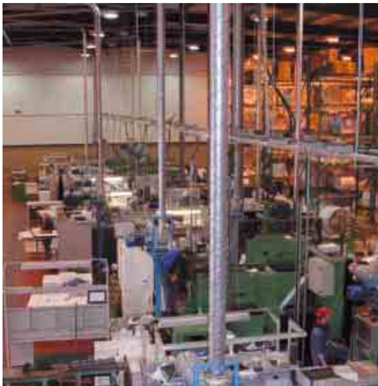
Spiral ducting takes matrix waste outside the building
