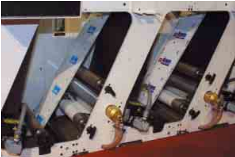
Web path on FBZ4200 allows 180deg chill roll contact
