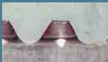
Cotron's eXact technology, Note symmetrical shoulders with 30 degree angles matching CTP
