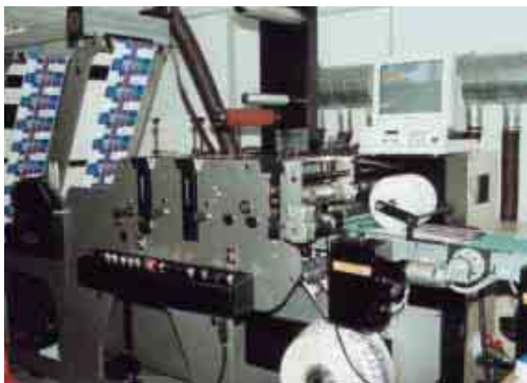
Die station converting cartons on the Beta press
