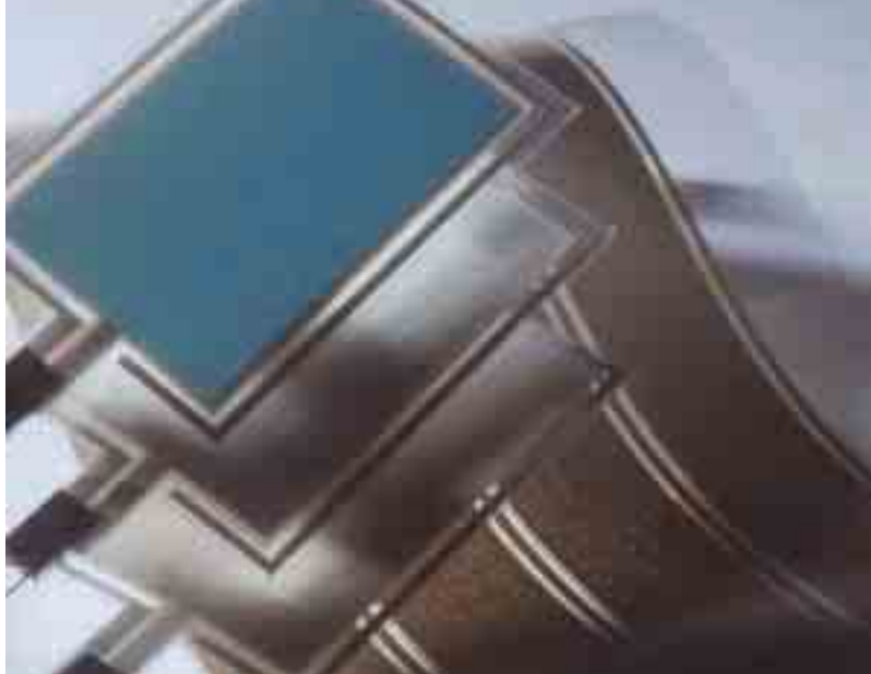
Ultra thin 'lamps' can be screen printed
