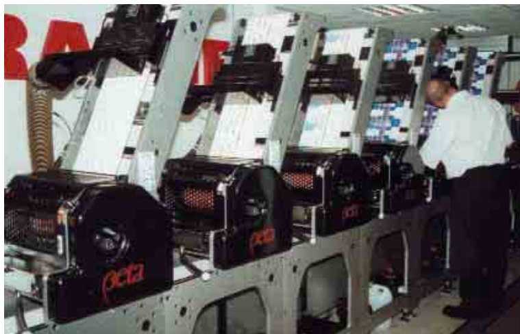
Cartons converted on a standard Edale Beta press
