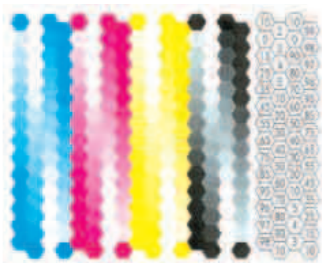
In a banded anilox roll trial, non-overprinting gray scales are used for all four process colours, showing dot gain expected during the print process
