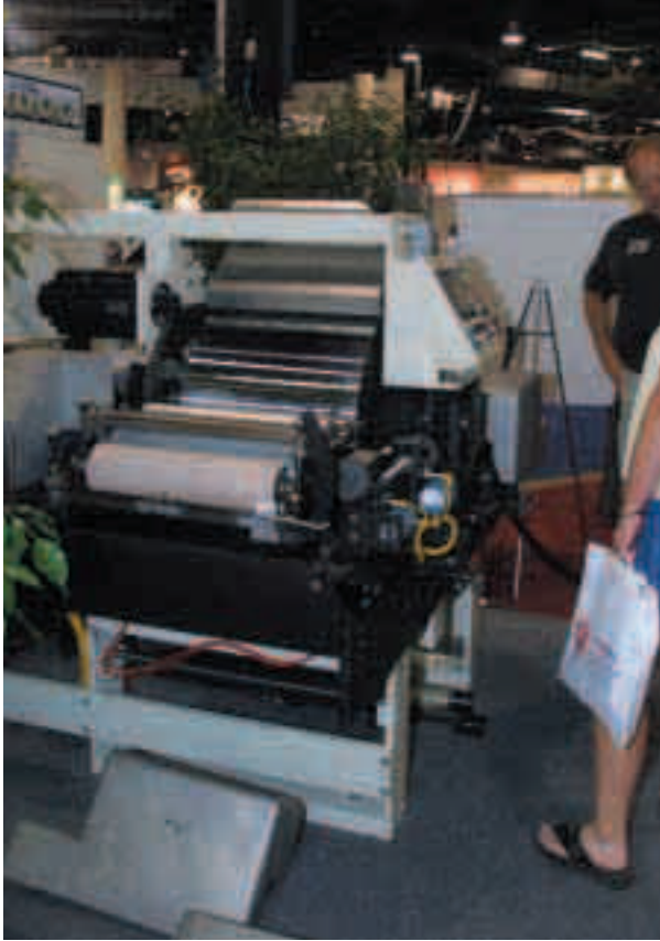
PCMC Deckx2 print module. Note CI drum between two print decks
