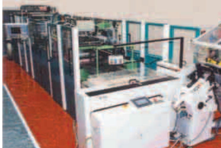
Womako strip cutter interfaced to Blumer counter pressure punch
