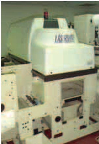
Fig. 3: A laser digital converting module, such as the LasX Industries LaserSharp, includes a sealed CO 2 laser, a high-speed motion system, and process control software.
