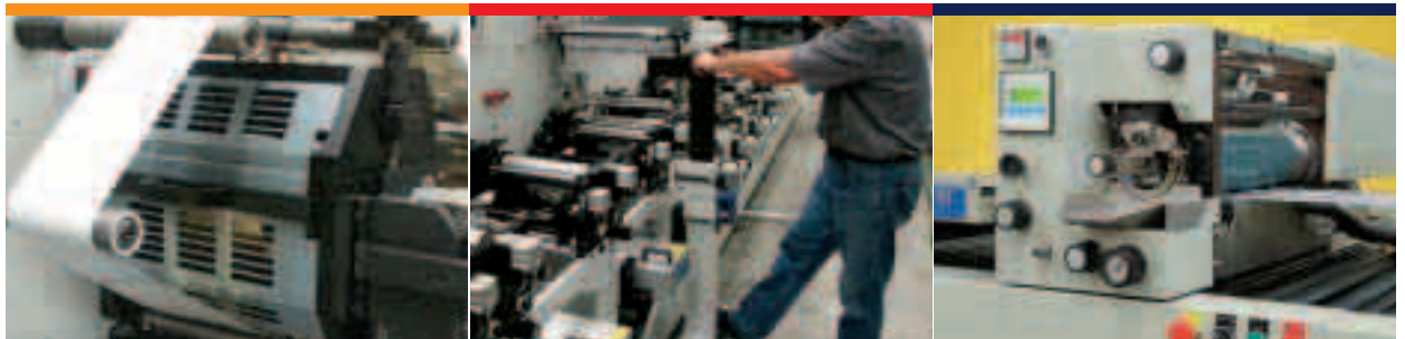
GiDue 'Ready' hot foil unit (left) and silk screen unit (centre). Silk screen module on Codimag Viva 340 press (right)
