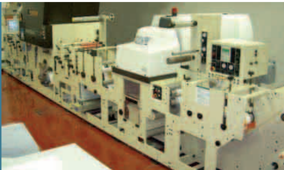
Fig. 1: All-digital label printing and converting system, the Mark Andy DT 2200, requires no plates, no dies and no make-ready time, because it incorporates four-color process digital ink-jet technology, as well as digital CO 2 laser converting technology.
