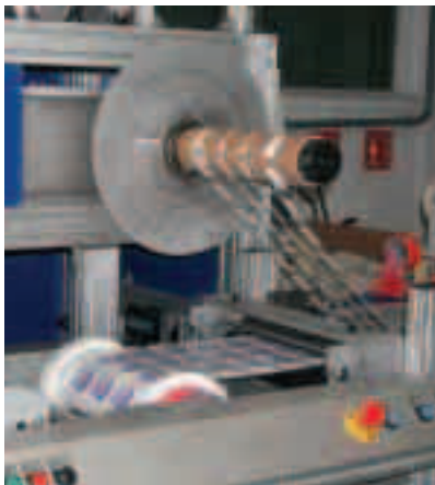
(above/below) After being offset printed, booklet labels have a pressure-sensitive backing liner applied by the Flytec system
