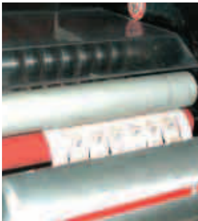
(above/below) Promotional labels being processed on the Prati Jupiter TC400 slitter rewinder
