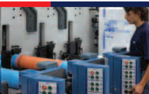
The Accordion control station on each print unit
