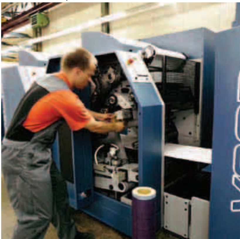
Changing sleeves during makeready on Drent Goebel's VSOP press
