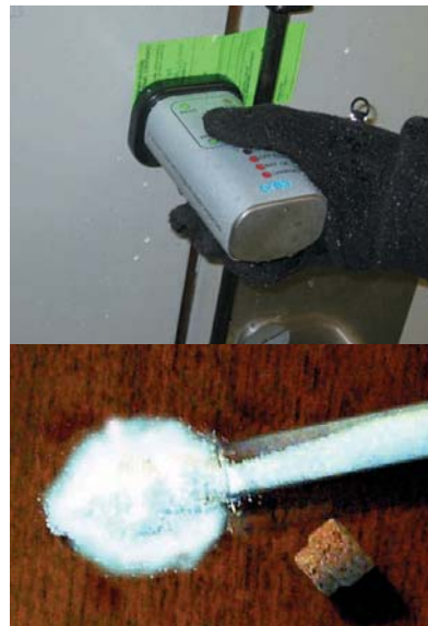
The dedicated reader unit (Top) can be used to identify the presence of the Traceless taggant particles (above)
