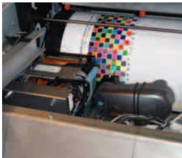
For the first time, DuPont includes an onboard GretagMacbeth spectrophotometer. It is standard on the Cromalin b3 and optional on the existing b2
