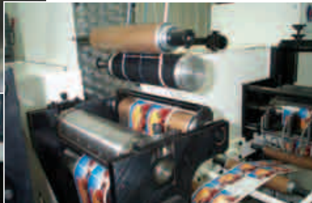
Left: print unit featuring quick set-up SAPS system (see box below), below left: Metronome press, below: Auto Peel-off allows waste stripping to start automatically
