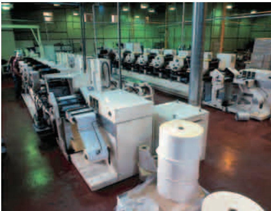
Parkers' facility in Aintree, Liverpool, houses three Nilpeter flexo presses and a Mark Andy 4200
