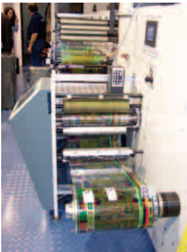
GiDue E-Combat UV flexo press applying Prime IT inline
