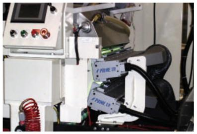
Prime UV's eight lamp FLEXfilm curing system
