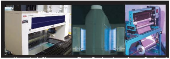
Enercon technology modifies surface tension of containers for correct label application
