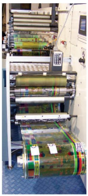
In-line application of Ciba's Prime IT coating on GiDue E-Combat press
