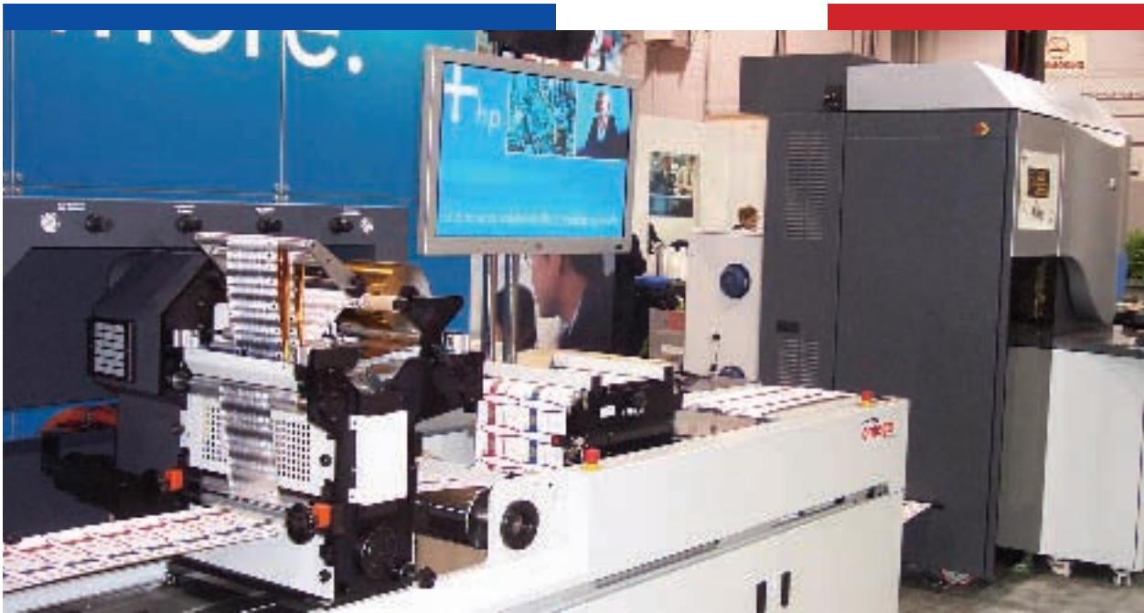
HP Indigo launched its ws4050 digital press with the ability to convert unsupported films including shrink film
