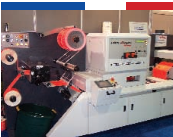
The Sabre Extreme laser die cutting unit
