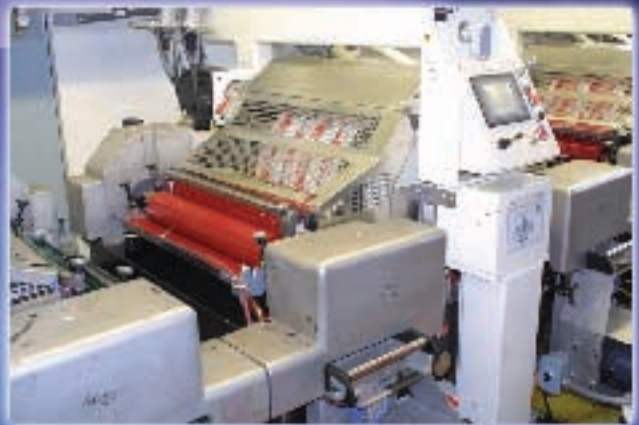
Modular Deck x 2™ design uniquely positions a print station on each side of a single impression cylinder.
