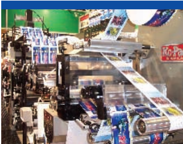
(Above) Complex film converting on Ko-Pack Flexo 400 press
