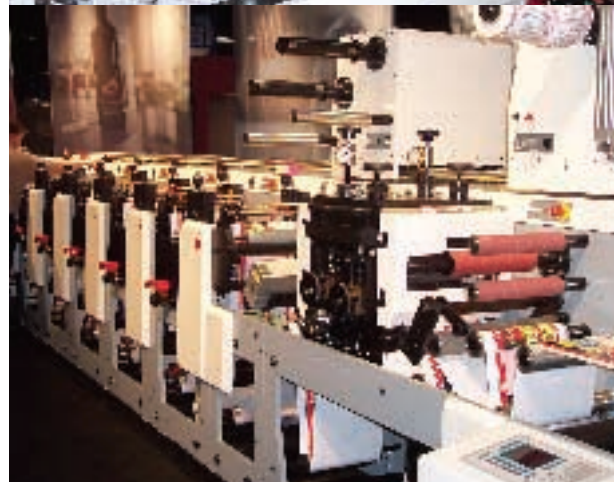
(Top) RFID tag affixing feeder from Longford intergrates with any web press. (Bottom) MPS EF 13" 6-color press
