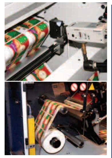
On the Digital Laser Workflow the ws4050 prints a barcode (top) which is read by the ABG converting line to control the laser diecut and motorised slit (below)
