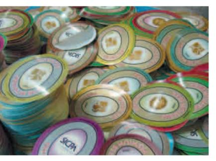
MetalFX can be used on labels to create multiple metallic colors all by using the silver base ink overprinted with CMYK
