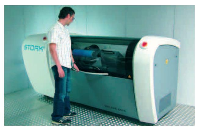
Stork's laser engravers can finish a typical plate for a label job in 20 minutes;
