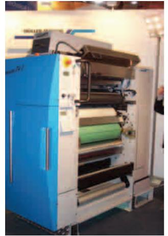
and waste, including pre-register and automatic washing cycle without the web running and a 'virtual' plate scanner for automatic ink key setting and memorizing jobs. Converting options include two die cutting stations and an embossing station. The press is available in 330 and 430mm widths.
