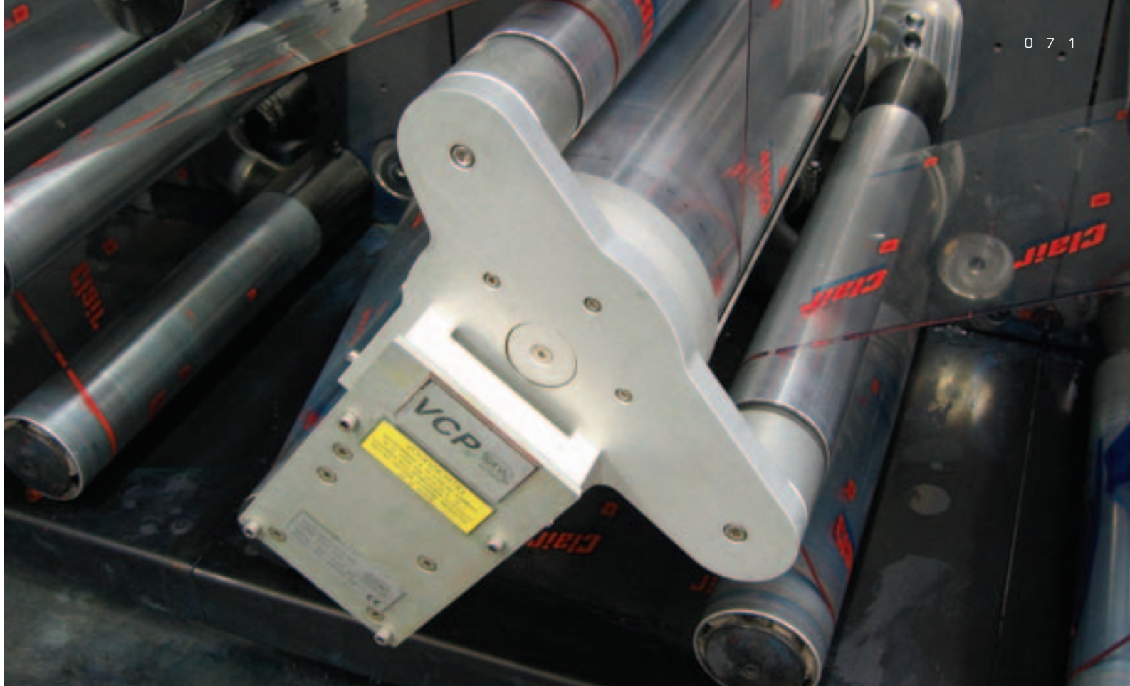
The GEW VCP-Film unit for UV curing heat sensitive substrates on presses without chill rollers
