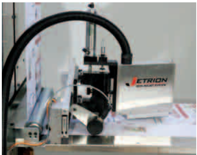
Mounted inline, the Jettrion 3025 adds variable data to labels
