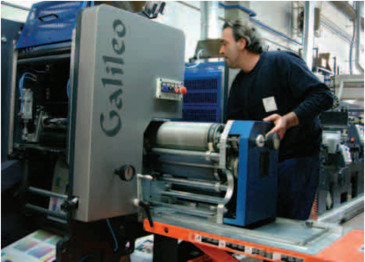
Exchanging print cassettes on the Castagnoli Galileo rotary UV offset press
