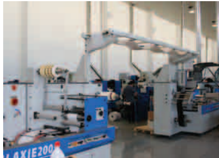
(Below) A bridge offers the opportunity to take the web through both screen presses
