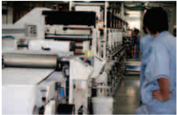
The 25 meter long Golden Gorges press is controlled by a new registration system
