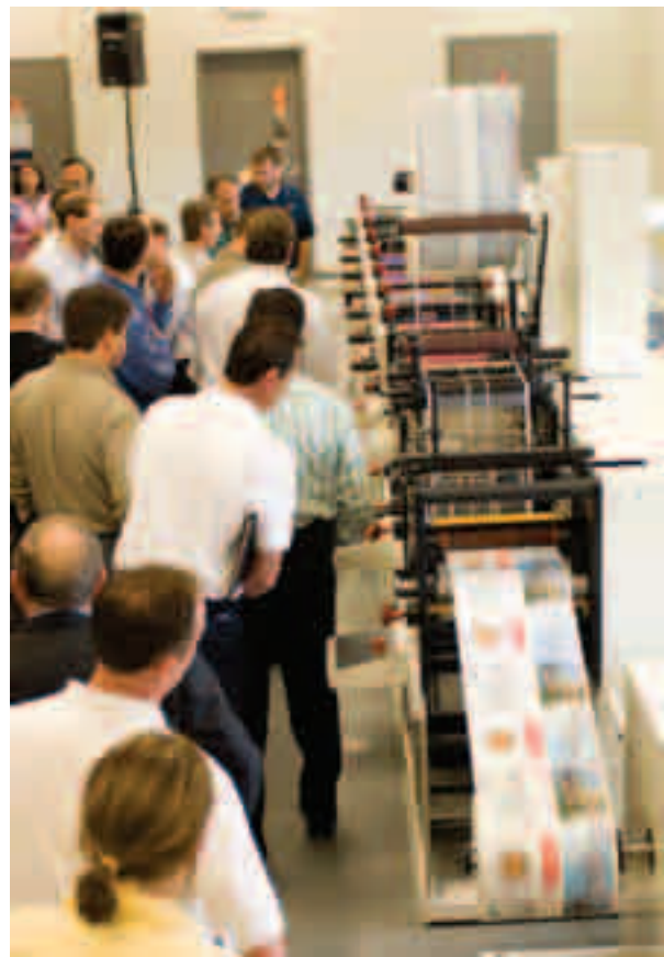
The Nilpeter FB3300A press printing a 200 line job with digital plates produced on a MacDermid LAVA thermal plate processing system
