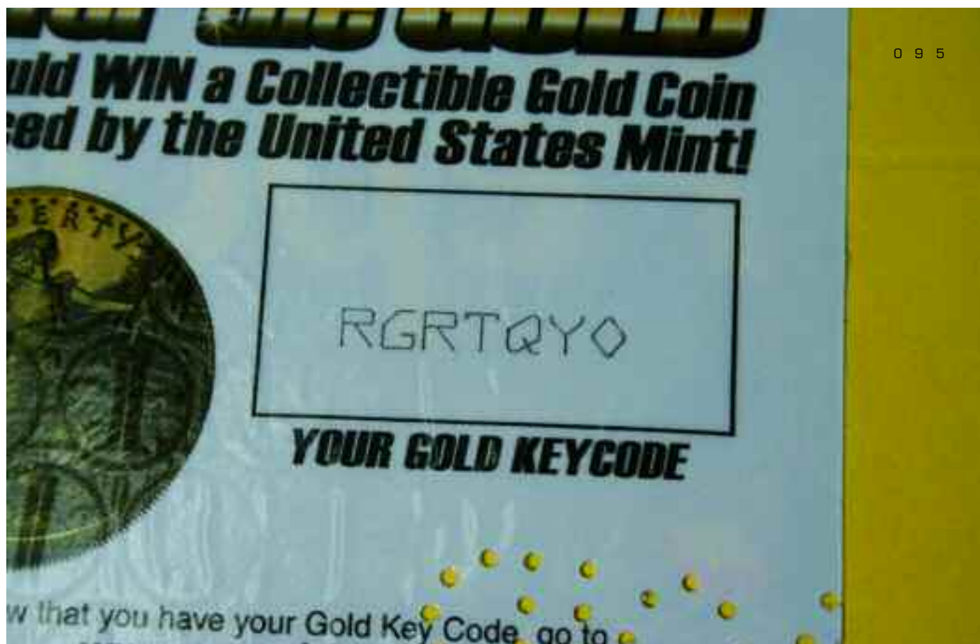
Under surface laser marking for security print applications
