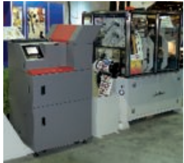
Newfoil model 3500/5500 hot foil and die cutting 'cool fusion' system
