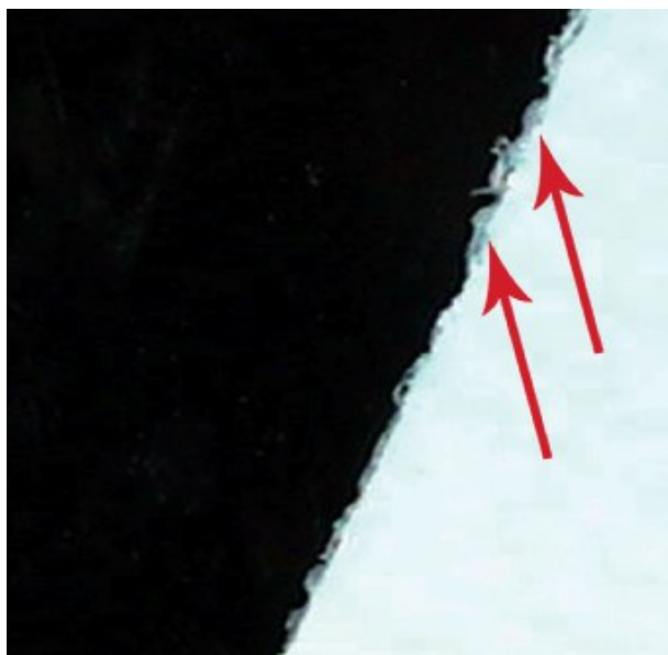
While light adhesive particles can be recognised in figure 5, which run out on the side under the label, figure 6 shows unproblematic material for comparison.
