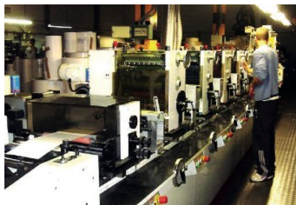
A 6-color semi-rotary offset press from Etipol from 2001, one of the many used presses that Grupoflex offers
