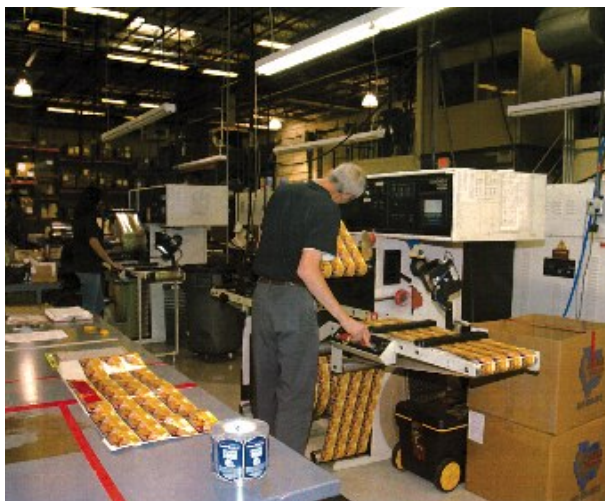
The use of Arpeco and Rotoflex inspection rewinder machines to standardize finishing operations
