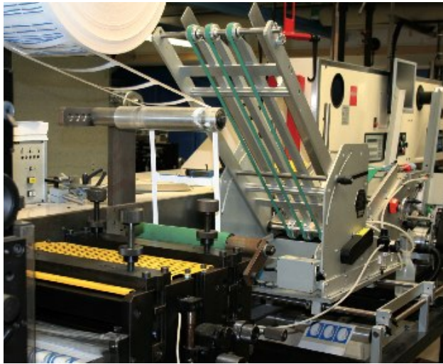
The Longford booklet inserter mounted on a Nilpeter B-3000 press
