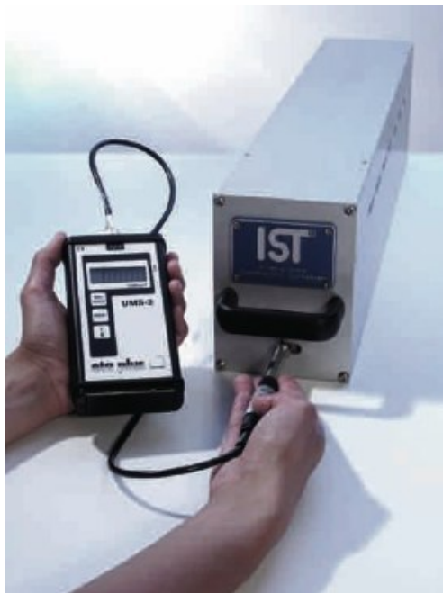
IST's UMS-2 is a typical portable device for measuring UV outputs
