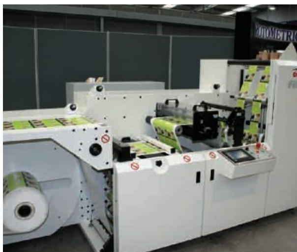
The Omega Filmic rewinder dedicated to handling unsupported materials
