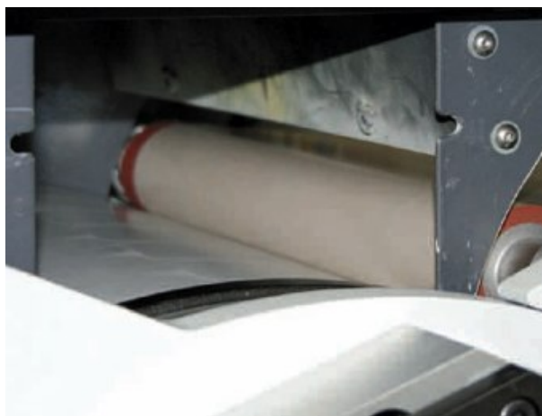
Delaminating the digitally printed web and laser die cutting on the backside of the label face before re-lamination
