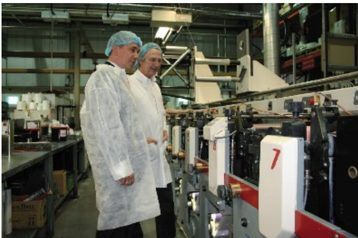
Harlands moved into UV flexo with this 330mm wide MPS press
