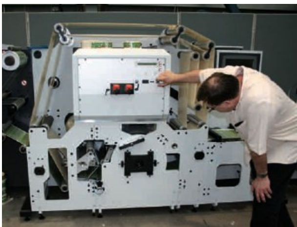
Delaminating the digitally printed web and laser die cutting on the backside of the label face before re-lamination
