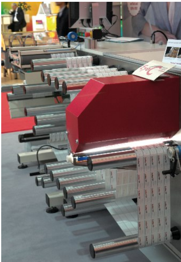
The inline EyeC ProofRunner combines 100% inspection with content verification
