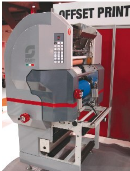
Codimag's Viva 420 featured the Aniflo keyless inking system
