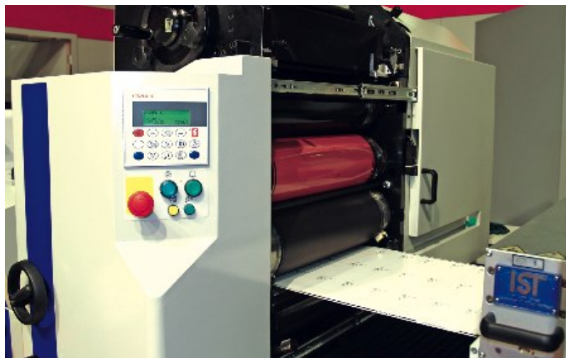
Codimag's Viva 420 featured the Aniflo keyless inking system
