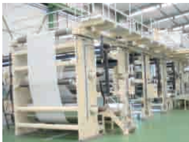
The new, tailor-made BMB automatic reel-fed coater
