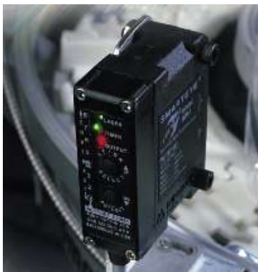
Laser sensor picks up invisible marker in ink
