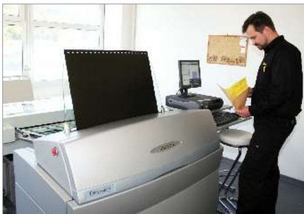
Imaging the Anthem Pro plates on Presstek's Dimension CTP imager
