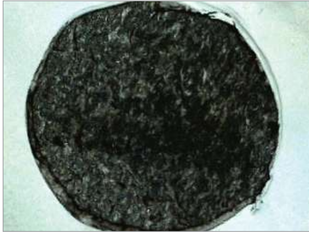
Picture of the surface after tearing off the bond
