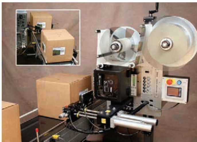
WEBER'S new Model 5300, shown in twin air-tamp mode, also offers an RFID printer-applicator option
