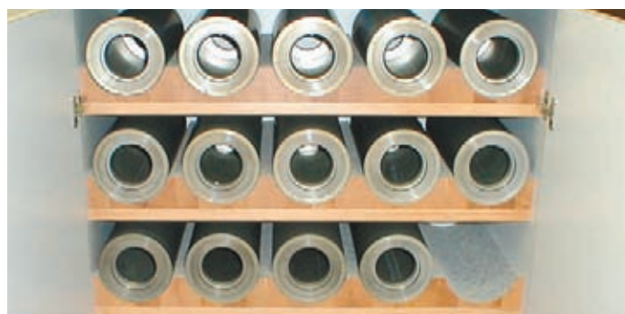
A TIDY WORK area and proper storage systems for plate cylinders and anilox rolls are critical elements in an efficient flexo workflow
