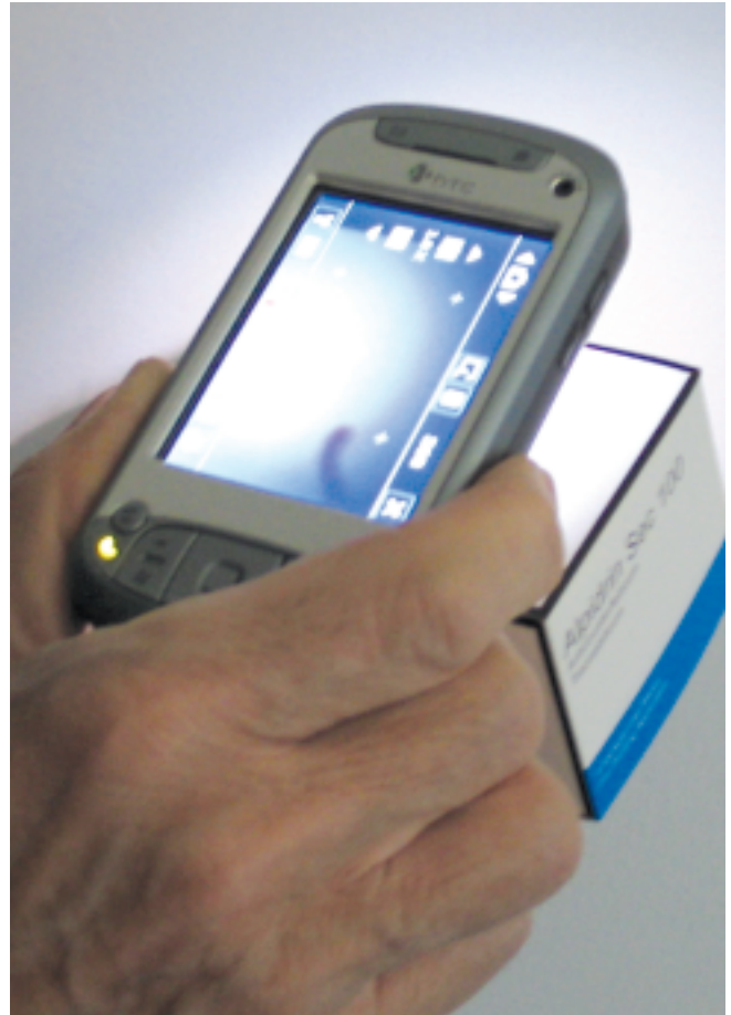
FIG. 4: PDA DIGITAL CAMERA USED TO AUTHENTICATE THE PRESENCE OR THE ABSENCE OF THE CRYPTOGLYPH INVISIBLE MARKING
