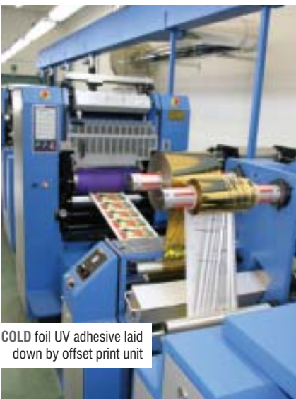
THE first four print units on the Rotatek Brava can be swapped between semi- and full rotary modes
