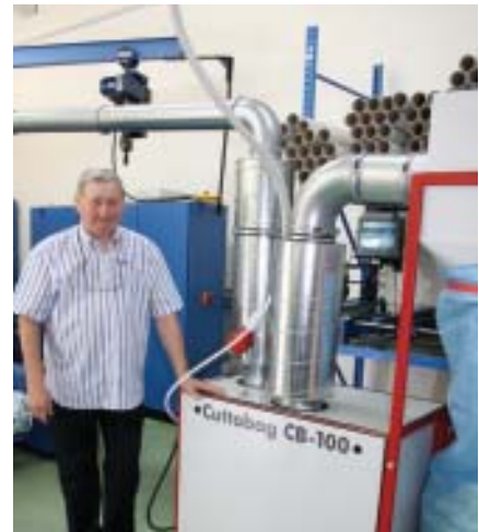
ZARDINI production director Tecchio Luciano demonstrates system which cuts up matrix waste and sprays it to kill adhesive
