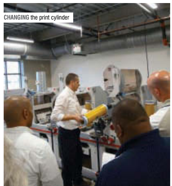
QUICK changeovers are possible with the slide-out ink unit cassette systems that allow for simple anilox changes
