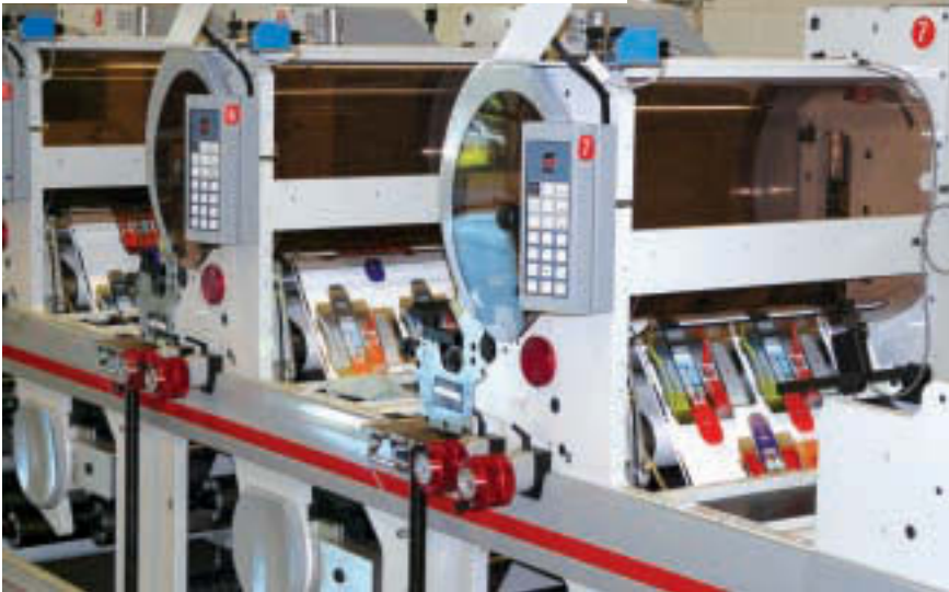
CLEMSON'S Omet Varyf ex has a 32in repeat chill drum for multi-substrate flexibility and a donated GEW UV e-brick system at each station
