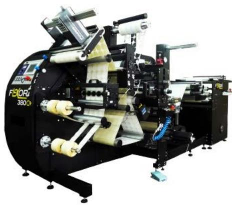
Flexor Jumbo: 280-520mm web width, 40" Jumbo Unwind, Double Die cutting, Re-Register, Fully S-Drive
