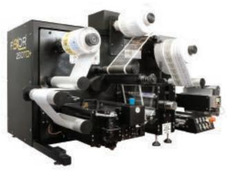
**Flexor 250TD:** 10inch wide converting and die cutting machine for small runs and re-register functionality.
