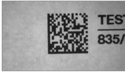
DIAGRAM 13: ILLUMINATION VERSION 3 . MODULATION GRADE 4 (VERY GOOD)
