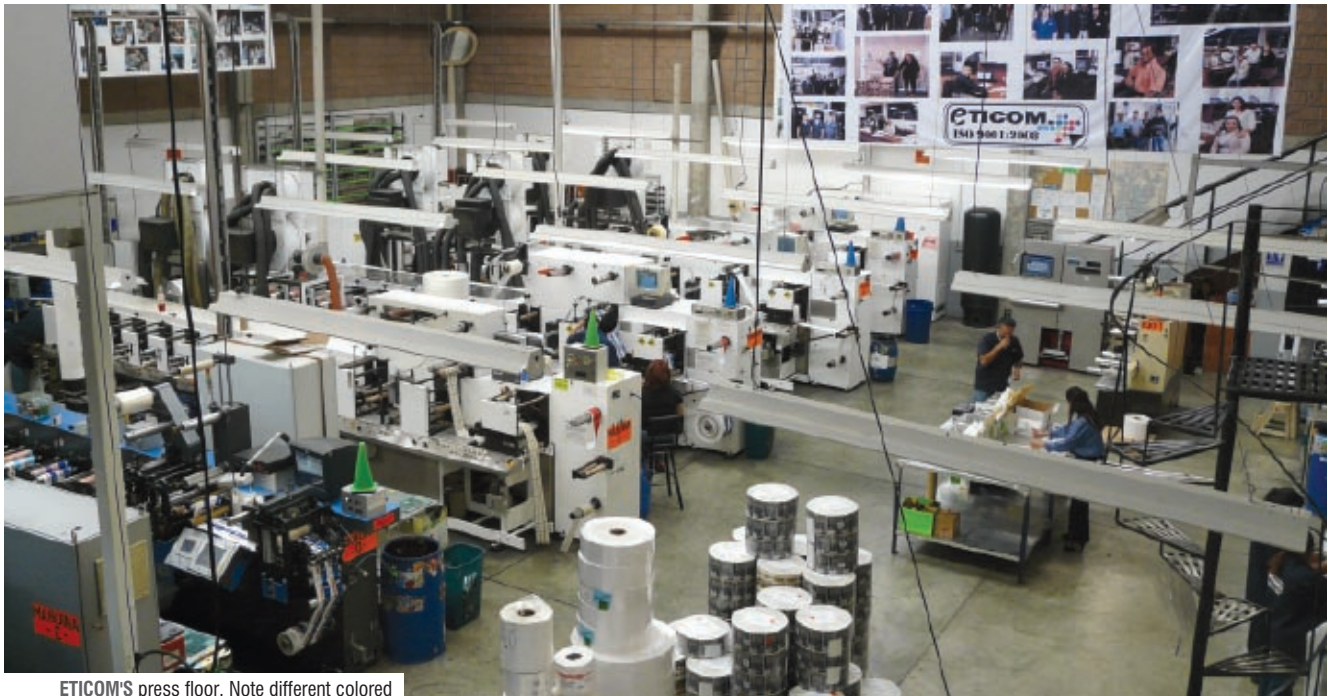
ETICOM'S press floor. Note different colored cones on ends of presses designating press status
