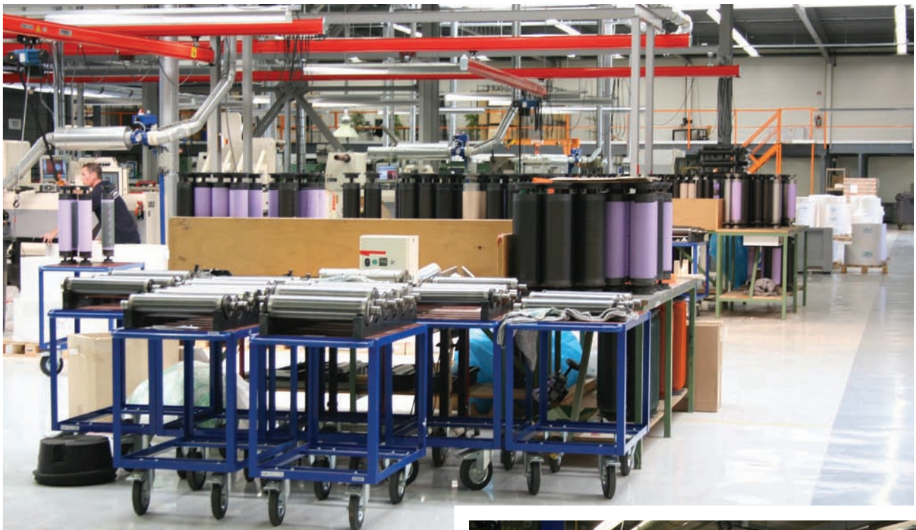
LEAN WORKING – well organized cylinder storage and delivery systems. Note also hoists (red bars) for moving heavy tooling to the press and Matho matrix removal ducting
