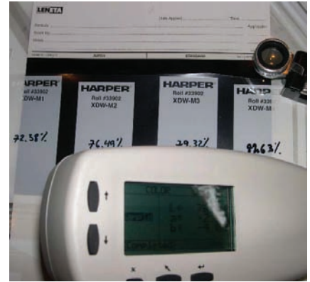
USING A SPECTRO-DENSITOMETER to measure opacity levels on site
