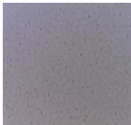
MEDIUM DUROMETER stickyback with HARD durometer polymer
