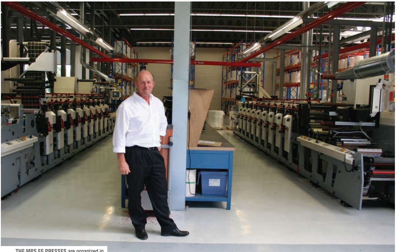
THE MPS EF PRESSES are organized in banks of two, manned by a three-strong team
