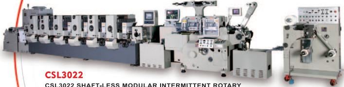
CSL3022 SHAFT-LESS MODULAR INTERMITTENT ROTARY LETTER-PRESS LABEL PRINTING MACHINE
