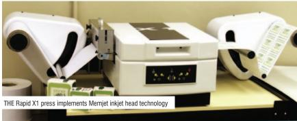
both machines to deliver in excess of 70 million drops of ink per second through over 70,000 nozzles.
