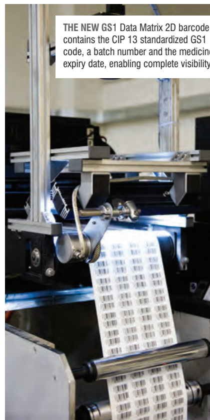
100 PERCENT BARCODE verification in action on a high speed variable barcode press used for pharma labeling
