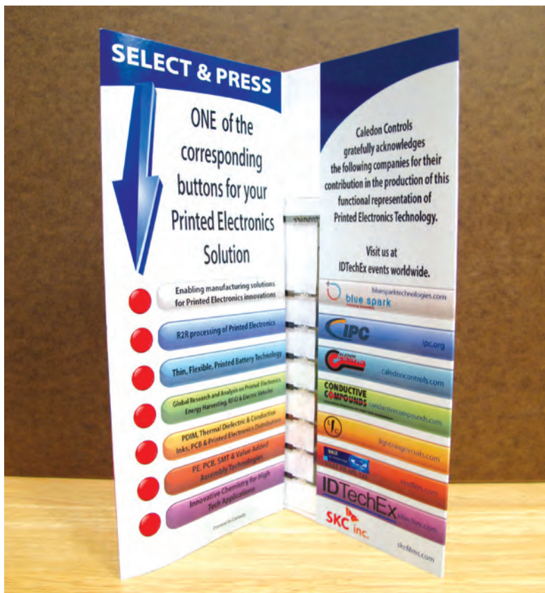
THIS demonstration brochure, which was distributed to attendees of Printed Electronics Europe 2012, provides a functional representation of printed electronics technology. The electronic components included microcircuits and mini LED lights powered by Blue Spark printed batteries. The photos show the brochure's front and inside, as well as an interior close-up of the embedded electronics
