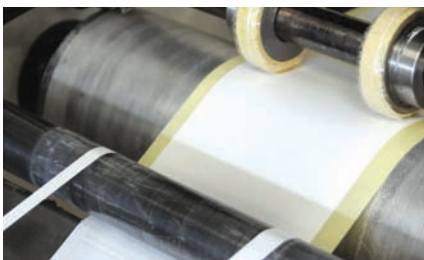
CLEAN REMOVAL OF CUTTING WASTE: In view of guaranteed adhesive application tolerances of just plus/minus one and a half grams, Hagmaier operates the laser die-cutting machine for paper labels only with Herma adhesive material.
