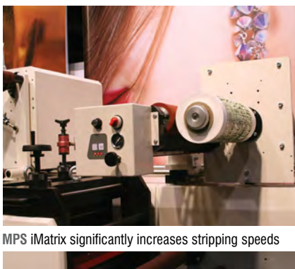
MPS rail-mounted die-cut unit with APC servo pressure
