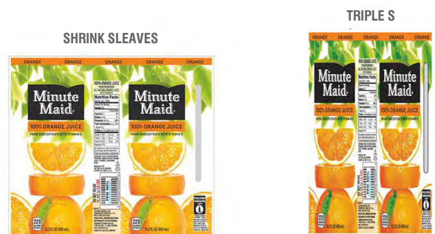
FIGURE 1: EXAMPLE OF TRIPLE S STRETCH SLEEVE PROVIDING LESS FILM WEIGHT PER SLEEVE WHEN COMPARED TO A SHRINK SLEEVE
