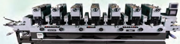
NEW SEN SPM300 / 320 / 350 (2,3,4,5,6,7,8,9,10 COLOURS + FLEXO VARNISH) JAPAN SPEC.
