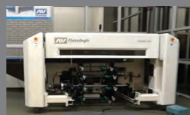
AV Flexologic FAMM HS machine for automatically mounting flexo and letterpress plates on cylinders/sleeves. www.labelsandlabeling.com/label-tv/technology/av-flexologic-famm-hs-plate-mounting-machine
