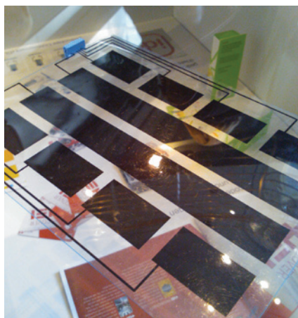
THE SURFACE OF SHELVES is equipped with printed electronics that complement those on the package and allow stock levels and other information to be communicated
