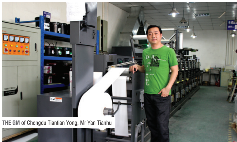
GIDUE M5-370 11-color press installed by Tianjie with 10 flexo printing units, 1 gravure unit and on-line process units including cold foil and turn bar
