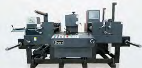
SEN SRD 360 Shaftless High Performance Intermittent Multi-Function Digital Label Converting Machine -Japan Spec Max. Paper Web Width:360mm Max. Converting Width:350mm Min / Max Repeat Length:30-370mm Die Cutting Speed:250 rpm
