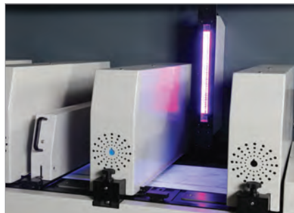
UV LED pinning for supporting optimal text and line definition
