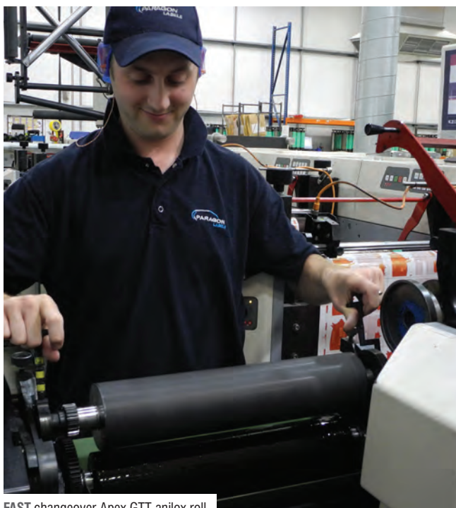
FAST changeover Apex GTT anilox roll
