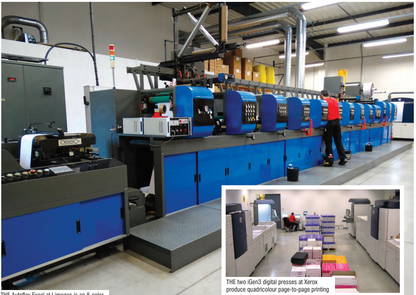
THE Autoflex Excel at Limoges is an 8-color flexo press with a 340mm web width
