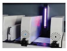
Unique LED curing after each color ensure crisp text, fine lines and maximise colour definition
