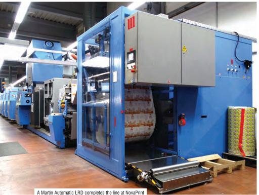
By combining up to 16 different jobs across the 850mm web, and slitting afterwards, NovaPrint can make better use of the new VSOP's performance on run lengths that are typically 10,000 -14,000 running meters per single roll. But, in making the runs lengths longer, with fewer machine stops, it needed to address the subject of waste control, and called in Martin Automatic to provide system solutions at the beginning and end of the press.
