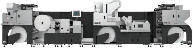
THE DIGICON 3000 is a 30in finishing system for pre-printed labels and flexible packaging
