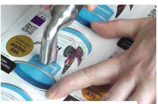
THE way curing is managed can have a huge impact on ink adhesion, and is something that can only be identified with proper scratch testing
