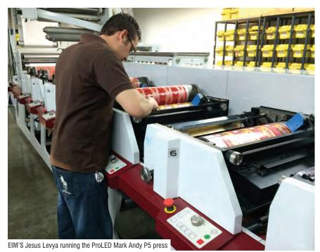
Stone explains, 'With ProLED on the P5 we don't often use the material chill rolls. Because of the low amount of heat produced from UV LED, there's no need to reduce the temperature of the material, particularly when printing on labelstock. Often we're using only the ProLED cooling system to maintain temperature consistency of the lamps.'
