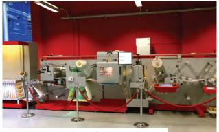
A Xeikon 3300 was shown with a DCoat 330 and inline laser die-cutting unit for the production of pharmaceutical labels
