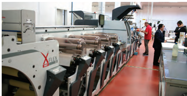
Four flexo units before the digital unit
