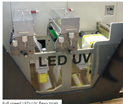
Full speed LED-UV flexo trials
