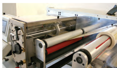
SmartCut automatic slitting knife positioning
