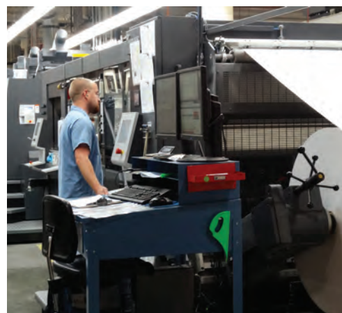
Left: One of Inland's latest nine-color Speedmaster XL 106 presses, fitted with coating units
