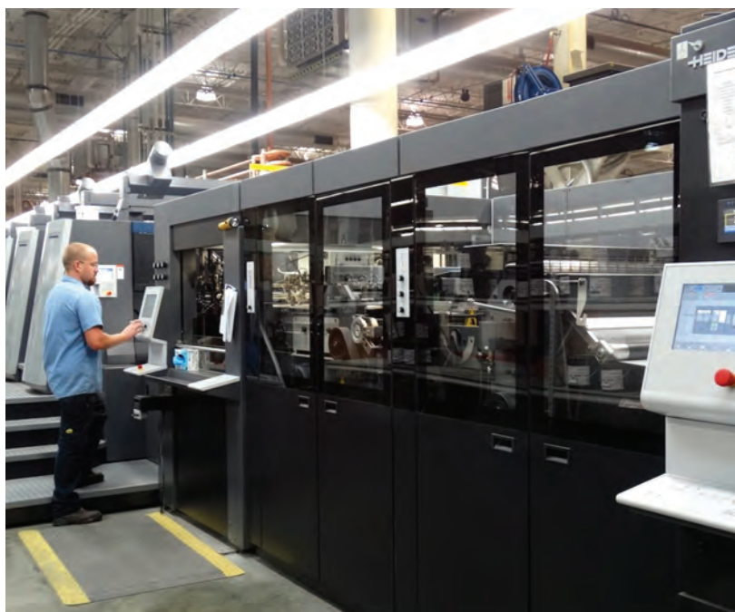
Left: One of Inland's latest nine-color Speedmaster XL 106 presses, fitted with coating units
