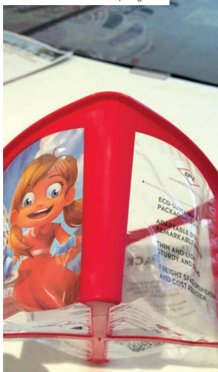
Precision Press produced laminated structure that works as both floor and wall of IML package
