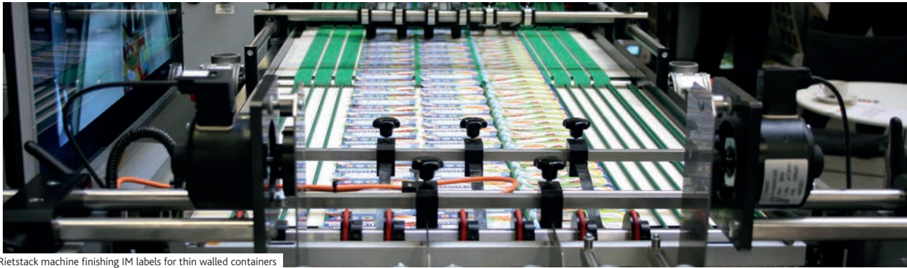
Rietstack machine finishing IM labels for thin walled containers
