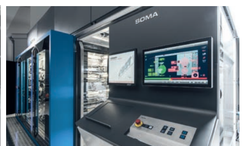
Available in 620mm (24in) and 820mm (32in) widths in up to eight colors, the Optima is capable of speeds up to 300m per min (984ft per min)
