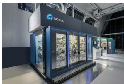
The Optima features unwind and rewind systems that are located outside the printing unit modules
