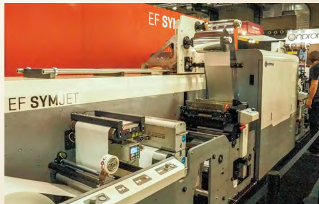
MPS EF Symjet incorporates Domino N610i digital print engine
