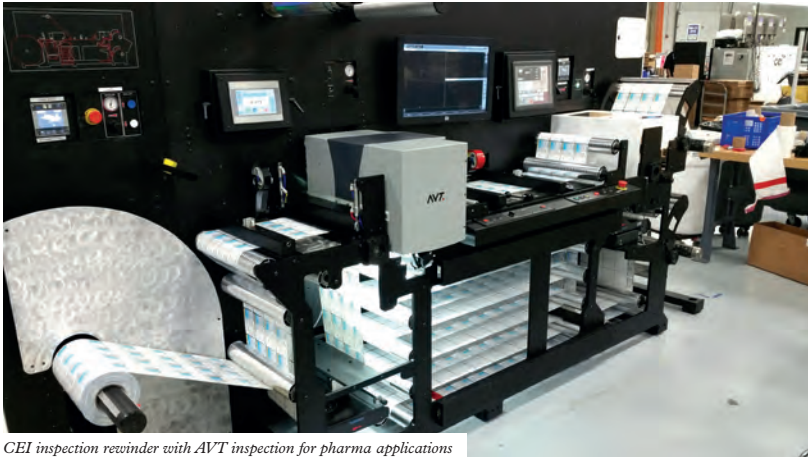
CEI inspection rewinder with AVT inspection for pharma applications
