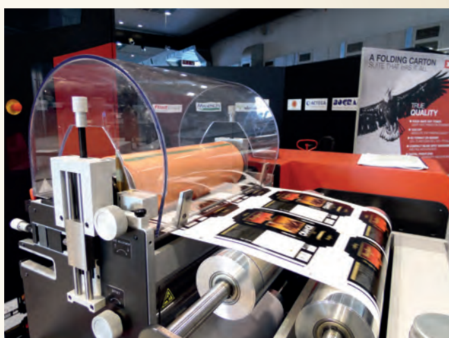
Roll-to-sheet digital folding carton production on a Xeikon 3500
