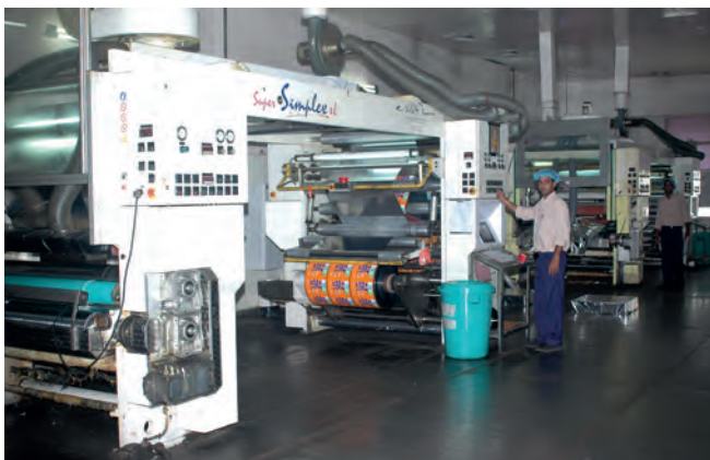
Solventless laminating machine at Uflex's packaging plant in Noida
