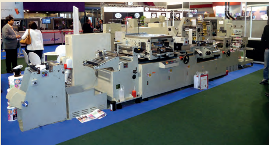
Orthotec launched the SRFD3030 finishing line for wine labels, incorporating a silkscreen printing unit
