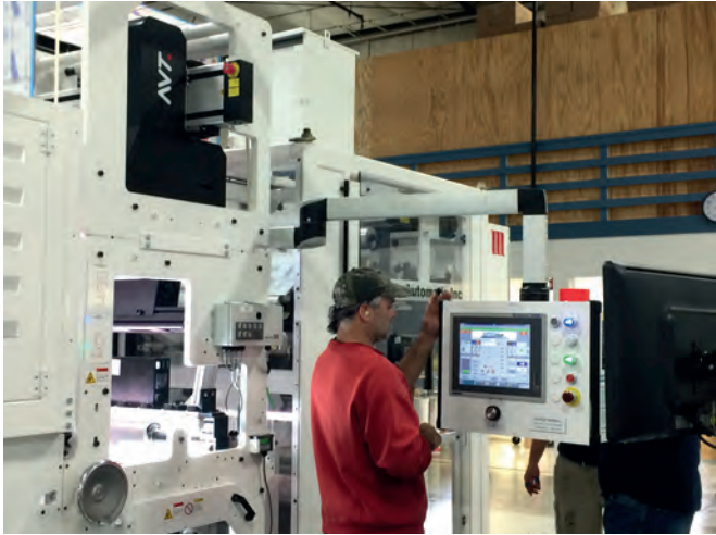
Full AVT inspection system and Martin Automatic turret rewinders
