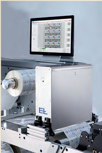
Erhardt+Leimer launched SmartScan, a camera-based quality assurance system
