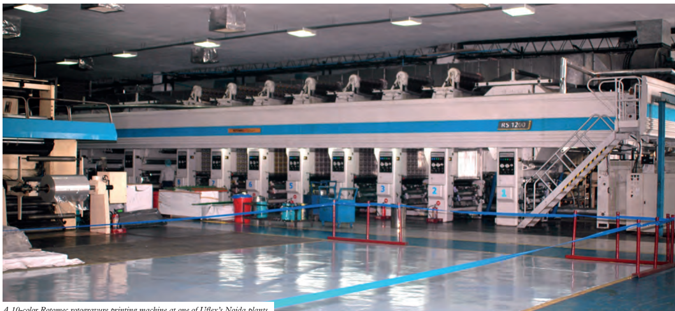
A 10-color Rotomec rotogravure printing machine at one of Uflex's Noida plants
