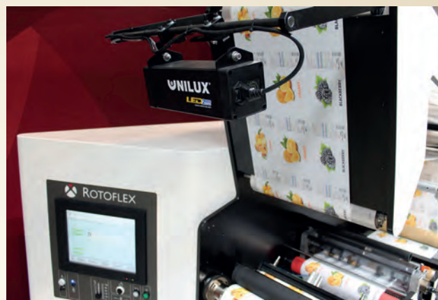
Rotoflex VSI and VLI slitter rewinders are now outfitted with the new Unilux LED-250 units
