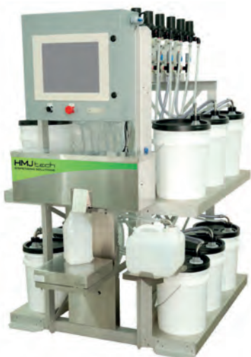
The HMJ-200 ink dispenser features a valve cluster that moves and indexes each valve to allow 'single point' batch dispensing into jugs
