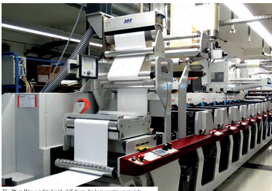
The P5 at Römer is fitted with chill drums for heat sensitive materials
