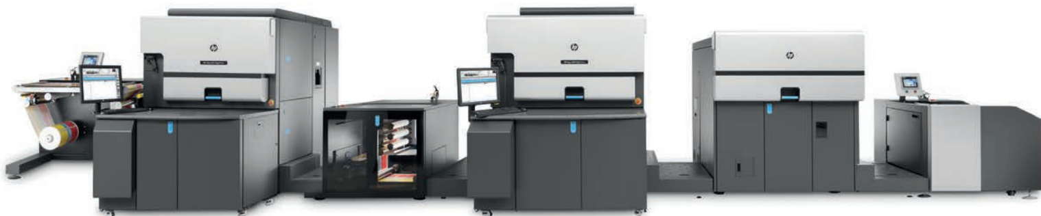
8000 press showing, from right, infeed, primer, master and slave print engines and connection for in-line converting
