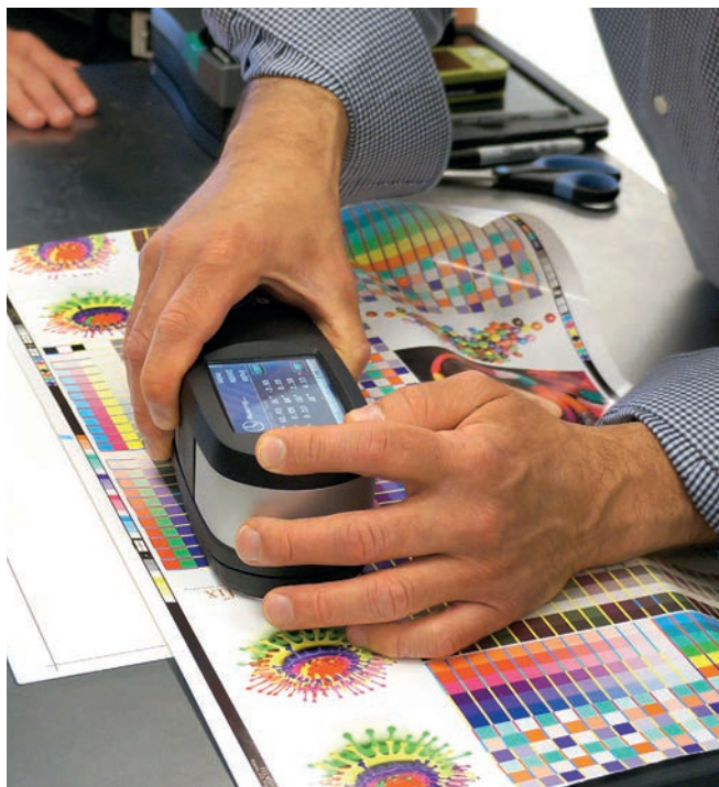
Performing a fingerprint test using a spectrophotometer to measure color and densities
