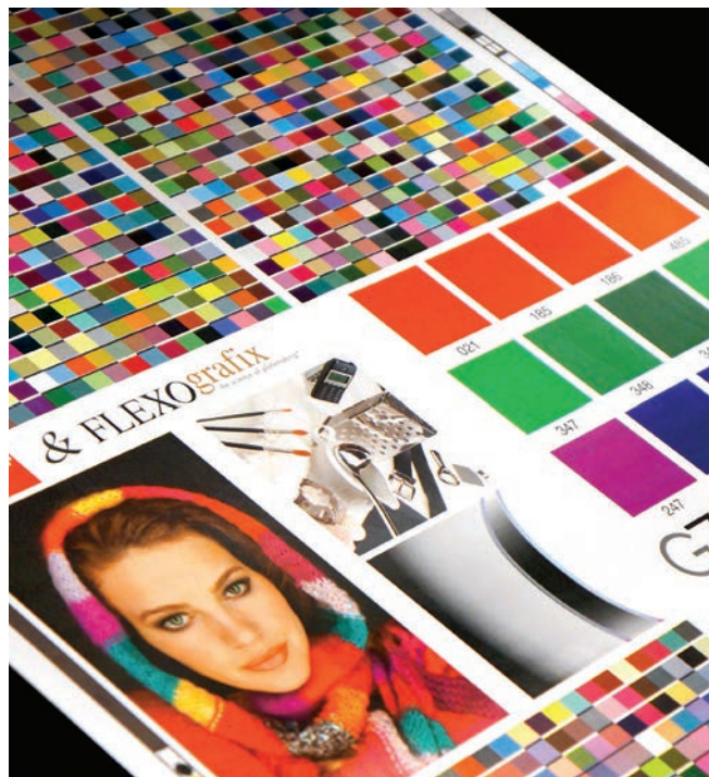
Profile test using a set of plates with the curve applied from the fingerprint
