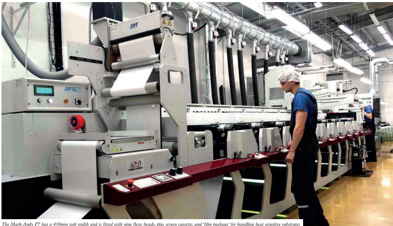
The Mark Andy P7 has a 430mm web width and is fitted with nine flexo heads, plus screen cassette, and 'film package' for handling heat sensitive substrates
