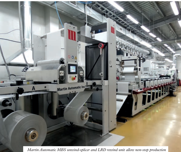
Martin Automatic MBS unwind-splicer and LRD rewind unit allow non-stop production
