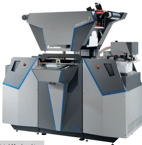
Leonhard Kurz's Digital Metal combines digital print with a metal transfer process
