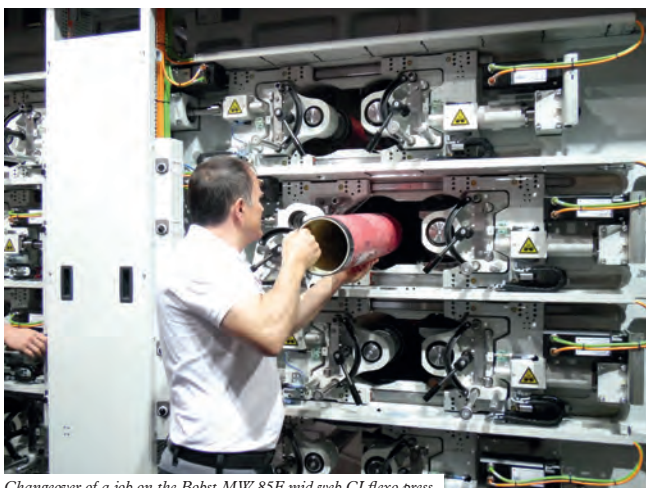
Changeover of a job on the Bobst MW 8SF mid web CI flexo press
