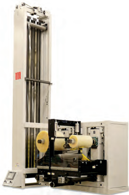
Martin Automatic's new MLSW splicer is designed for self-wound laminate film
