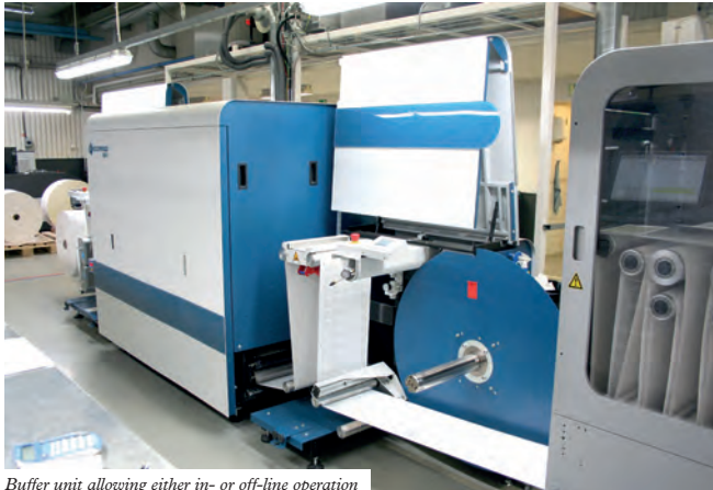
Buffer unit allowing either in- or off-line operation
